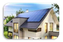
So, you will still need to buy electricity from the grid, especially on dark winter evenings. Our research and experience points towards the fact that a PV Solar Panel system is most effective when combined with a correctly sized battery, so that in the evenings, when energy consumption is highest and there is no sun, it [the home] can use the backup battery to supply electricity, as such significantly reducing the amount of electricity you need to buy from the grid.
